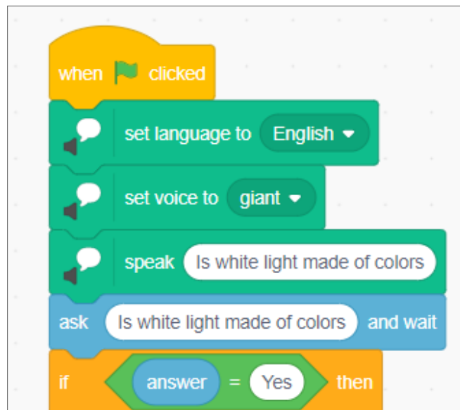
Figure 4.15. Screenshot from Kumari’s game showing the codes added to make the sprite both speak and produce a speech bubble.
